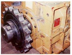
For the completed repair, no machining was necessary. Procedure saved owner considerable downtime as a new gear box would not be available for nine months
